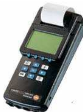
Figure 5.12 The control unit 350/454 [31].
