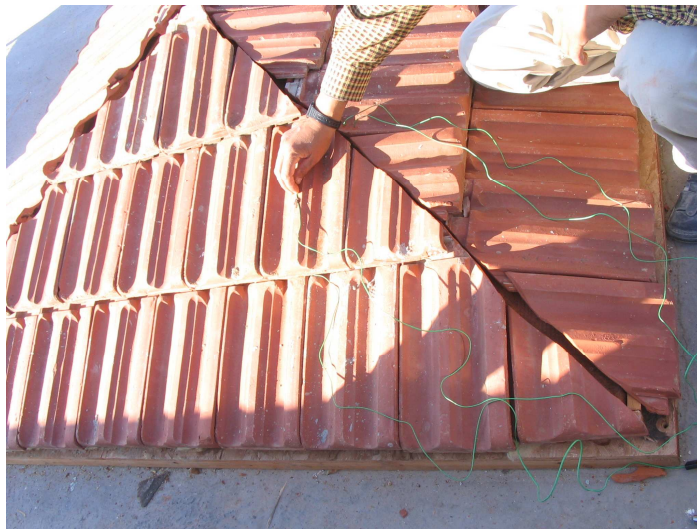
Figure 5.17 The roof tiles were put above the roof battens for both L1 and L2. Thermo couple cables were put to the layers of both hip roofs on their south facades.
